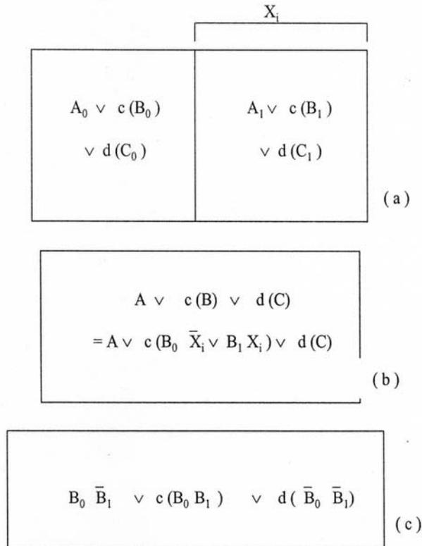
Fig. 1. Generation of a cell entry in the  $X_i$  VEKM in terms of cell entry/entries in the  $X_{i+1}$  VEKM : (a) pertinent cells in the  $X_{i+1}$  VEKM when  $X_i$  is a map variable, (b) pertinent cell in the  $X_{i+1}$  VEKM when  $X_i$  is an entered variable, (c) corresponding cell in the  $X_i$  VEKM.
