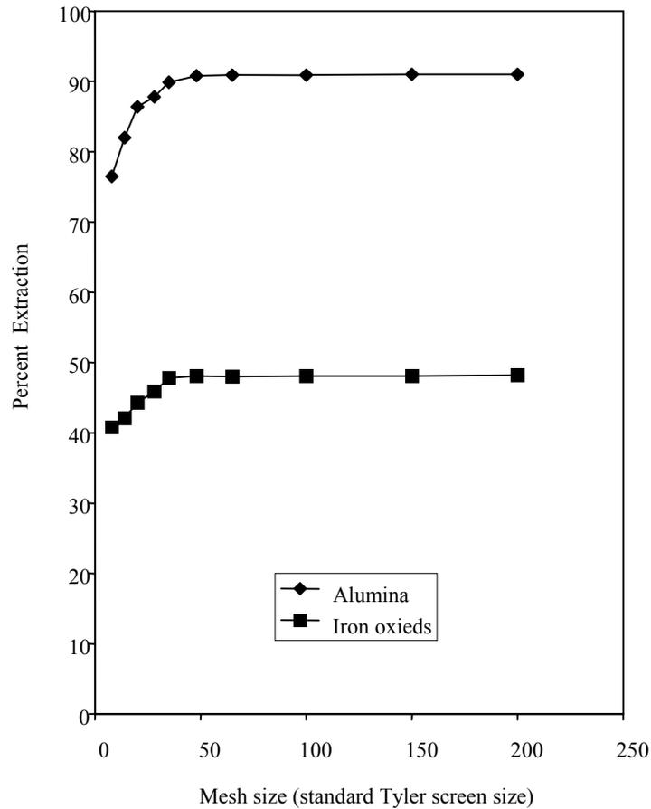
Figure1. Effect of grain size on percent extraction. Calcination temp. 700 ° C for 1 hr. leaching with 40% by wt. H<sub>2</sub>SO<sub>4</sub> at boiling conditions and a grain size of mesh no. -65 (standard Tyler screen mesh).
