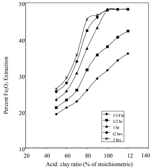
Figure 7. Effect of acid to clay ratio on extraction of  $\text{Fe}_2\text{O}_3$  at different leaching periods. Grain size: -65 mesh standard Tyler screens, calcination at  $700^\circ\text{C}$  for 1 hr and leaching with 40% by wt.  $\text{H}_2\text{SO}_4$  at boiling conditions.
