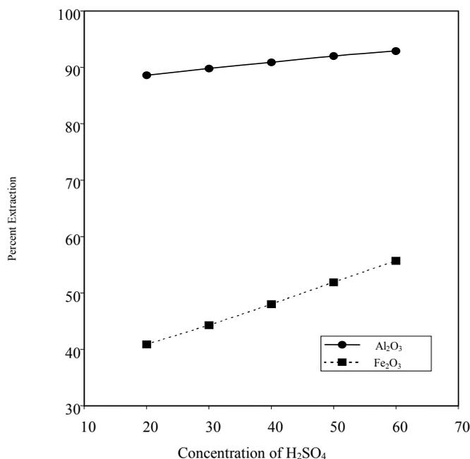
Figure 3. Effect of acid concentration on extraction of Al<sub>2</sub>O<sub>3</sub> & Fe<sub>2</sub>O<sub>3</sub>. Grain size: -65 mesh standard Tyler screen and calcination temperature at 700 °C for 1 hr.
