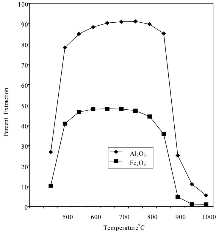
Figure 2. Effect of calcination temperature on percent extraction. Calcination time of 1 hr, leaching with 40% by wt. H<sub>2</sub>SO<sub>4</sub> at boiling conditions and a grain size of mesh no. -65 (standard Tyler screen mesh).
