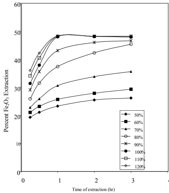
Figure 5. Effect of extraction time on % Fe<sub>2</sub>O<sub>3</sub> extraction at different acid to clay ratios.
