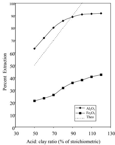
Figure 8. Effect of acid to clay ratio on extraction of  $\text{Al}_2\text{O}_3$  &  $\text{Fe}_2\text{O}_3$ . Grain size: -65 mesh standard Tyler screens, calcination at  $700^\circ\text{C}$  for 1 hr and leaching with 40% by wt.  $\text{H}_2\text{SO}_4$  at boiling conditions.
