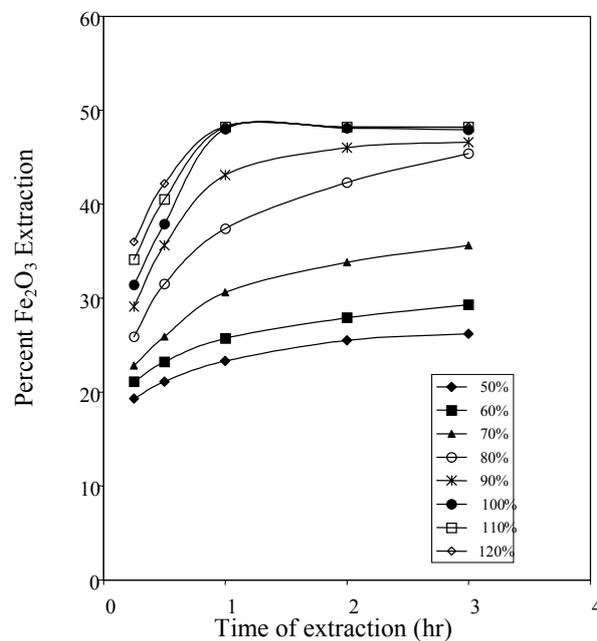
Figure 4. Effect of extraction time on %  $\text{Fe}_2\text{O}_3$  extraction at different acid to clay ratios.
