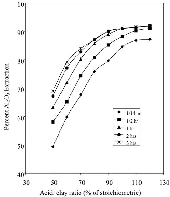
Figure 6. Effect of acid to clay ratio on extraction of  $\text{Al}_2\text{O}_3$  at different leaching periods. Grain size: -65 mesh standard Tyler screens, calcination at  $700^\circ\text{C}$  for 1 hr and leaching with 40% by wt.  $\text{H}_2\text{SO}_4$  at boiling conditions.
