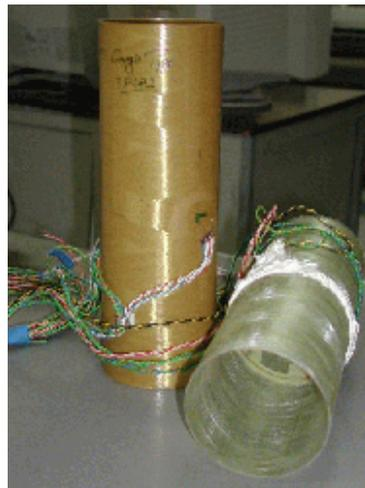
Fig. 11. Two tubes made from composite materials.
