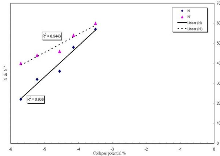
Figure 6. SPT before & after wetting (N & N') on the top of collapsible soils in function of collapse potential
