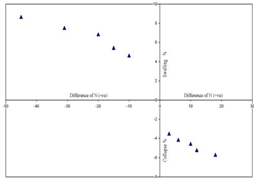
Figure 9. Difference of SPT values between dry and wet states correlated to swelling & collapse potential
