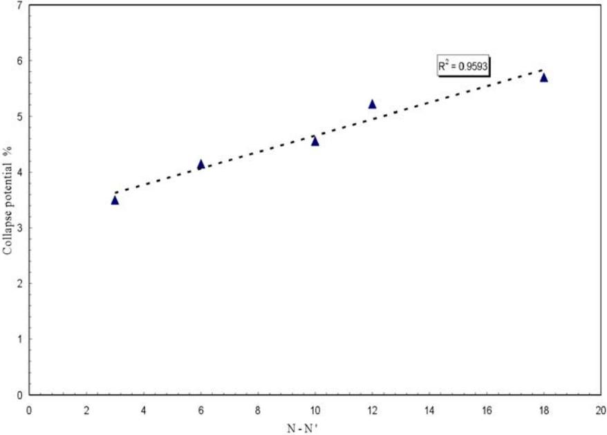
Figure 8. Collapse potential in function of the difference of SPT Number (N - N')
