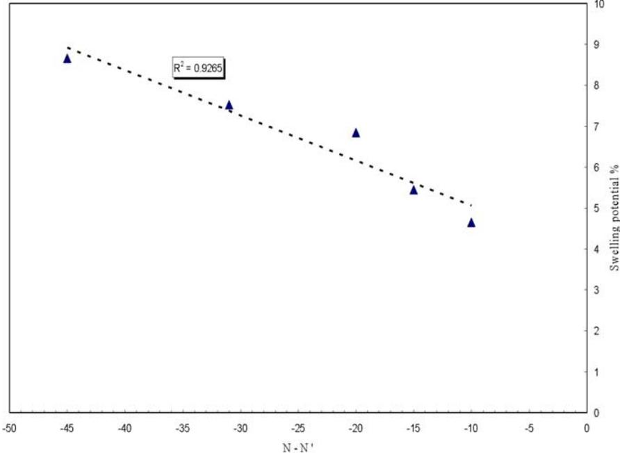
Figure 7. Swelling potential in function of difference of SPT Number (N - N')
