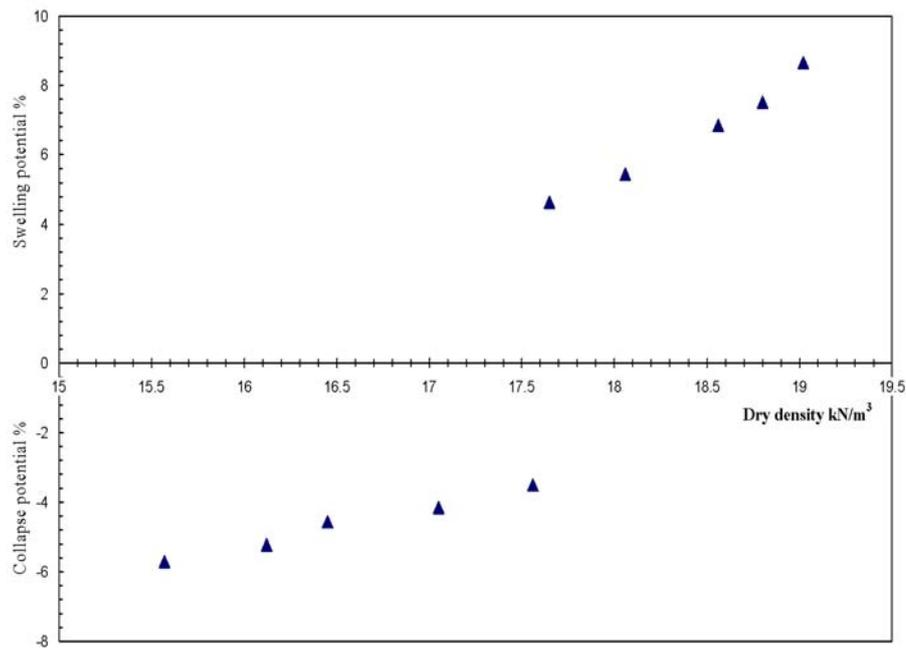
Figure 2. Swelling and collapse potential in function of dry density
