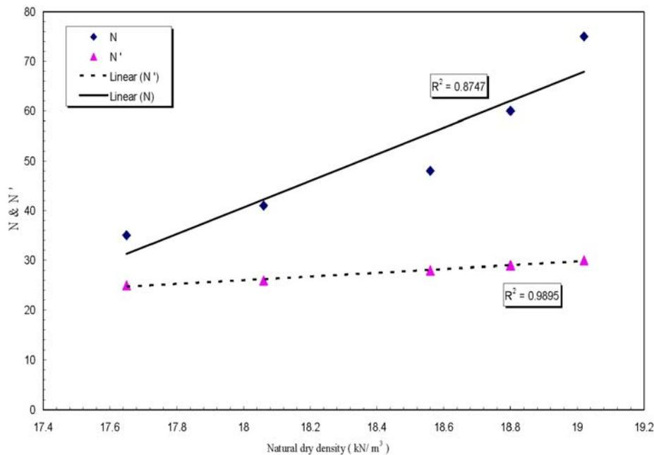
Figure 3. SPT before & after wetting ( $N$  &  $N'$ ) on the top of expansive soils in function of natural dry density
