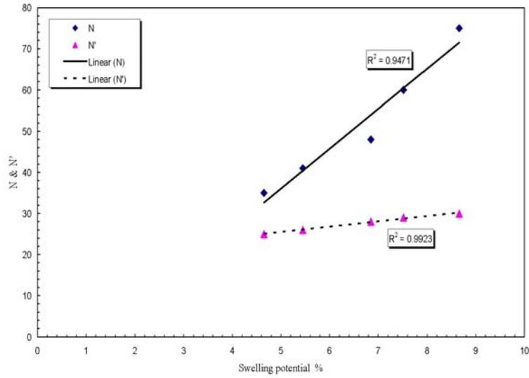
Figure 4. SPT before & after wetting (N & N') on the top of expansive soils in function of swelling potential
