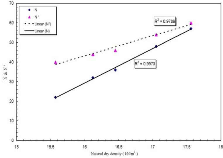
Figure 5. SPT before & after wetting (N & N') on the top of collapsible soils in function of natural density
